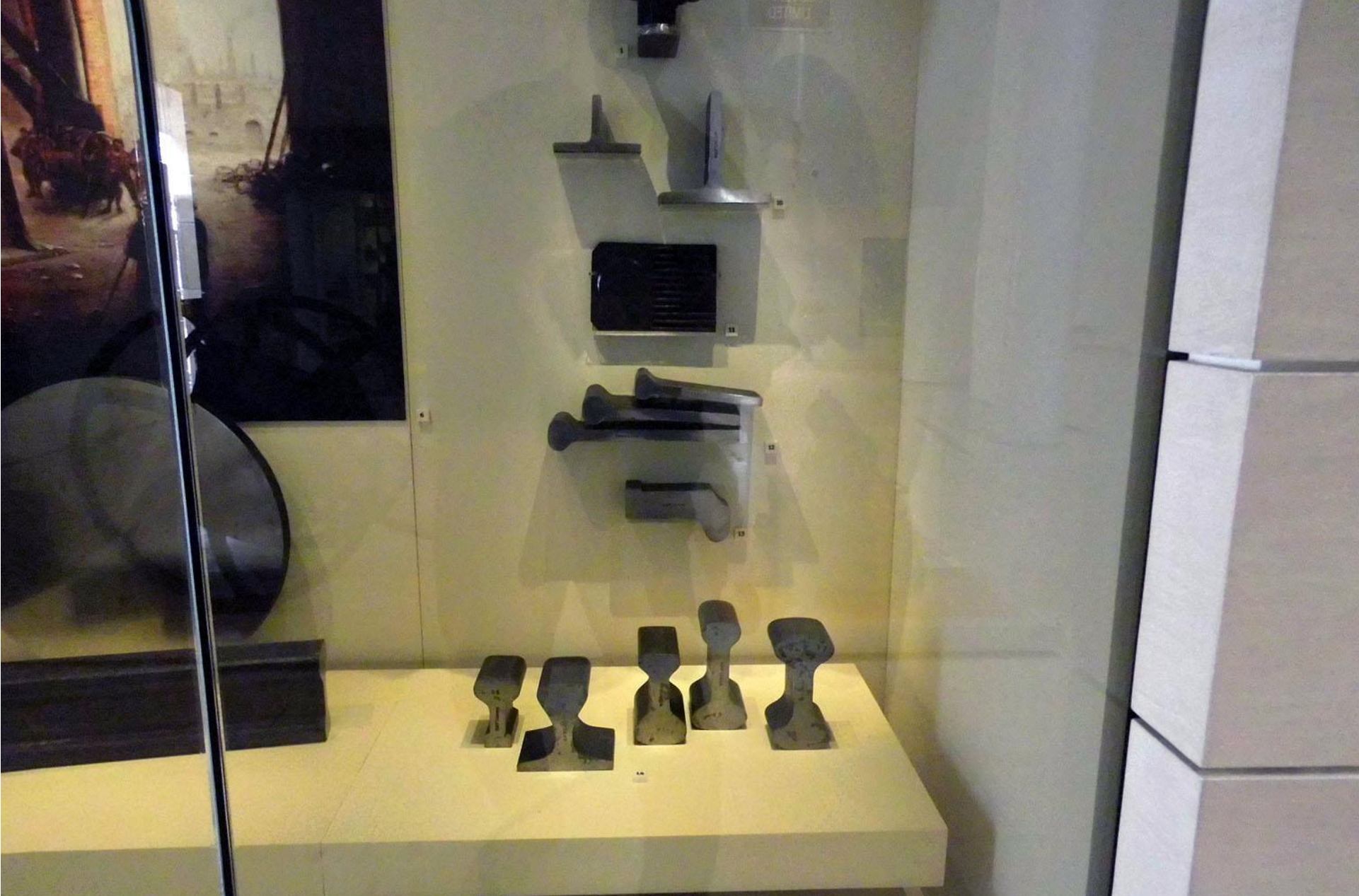
8 Slice cut from a wrought iron shaft, probably a ship's propeller and etched to show structure which is characteristic of wrought iron. 1850-1860 9 Sections of single-headed iron rails, made at Monklands Ironworks
